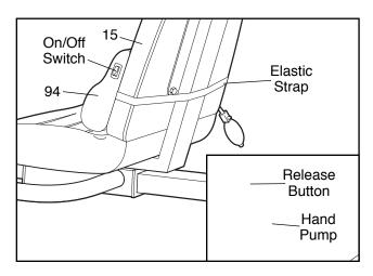
The firmness of the Lumbar Cushion (94) can be adjusted as desired using the attached hand pump. To increase the firmness, squeeze the hand pump repeatedly. To decrease the firmness, press the release button.
